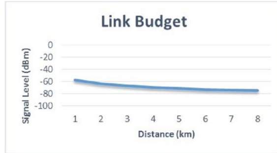
Fig. 5. Link budget calculation using Okumura-Hata model.
